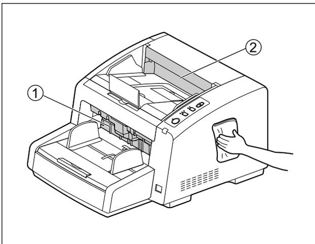
3. Remove dirt and dust from the fan exhaust vent (①) with a brush.
