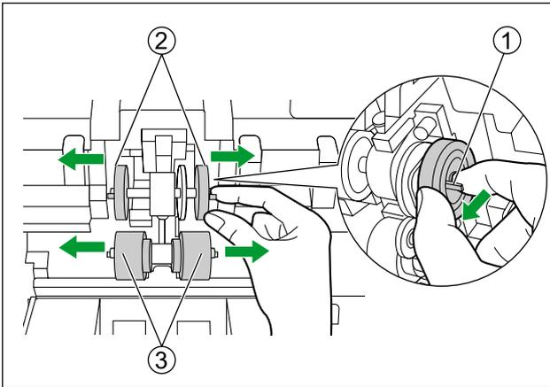
5. Take out the new paper feed rollers and separation rollers in the optional "Roller exchange kit (KV-SS033)".
