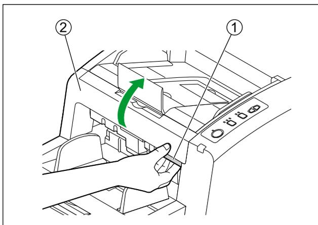
3. Move the reference plate lever (R) (①) and the reference plate lever (F) (②).
