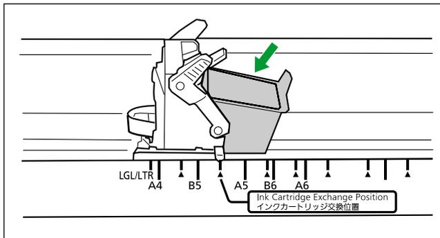
5. Lock the ink cartridge adjustment lever (①).
