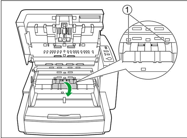
4. Remove the double feed prevention roller (①) in the direction of the arrow.
