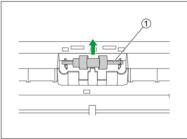
5. Take out the new double feed prevention roller in the optional "Roller exchange kit (KV-SS033)".
