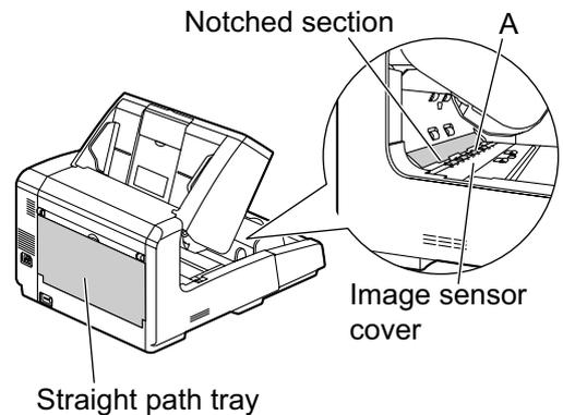
If the straight path tray is open, touching the notched section can cause injury.
