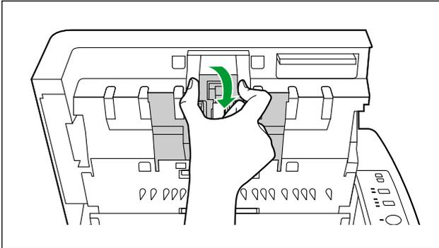
4. Turn the roller tip (①) towards you, and remove rollers from the shaft while opening the tip.
