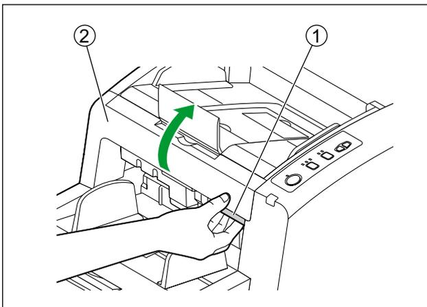
3. Remove dirt on the sensors with the included blower (①), then wipe the image sensor covers with the roller cleaning paper (page 48).
