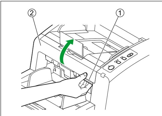
3. Pull open the double feed prevention roller cover towards you by using the indent (①).
