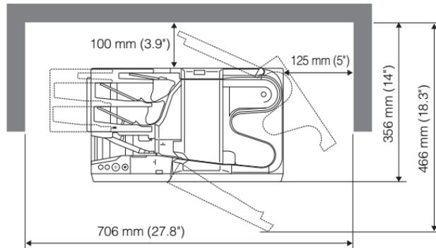
For operation, maintenance, and ventilation, make sure that there is enough space around the scanner, as shown in the illustration above.
