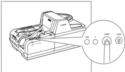
If the above procedure does not clear the paper jam, perform the following to remove the jammed document.
