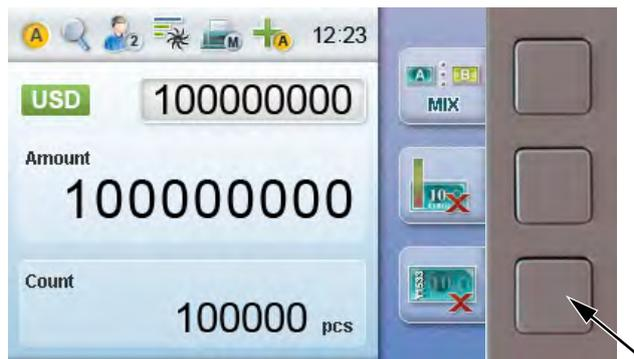
Figure 11: Enabling Serial Number, Ticket Reading or Check Function
