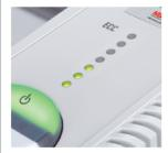
"ECC" (Electronic Capacity Control) indicator helps prevent paper jams by monitoring capacity levels during operation.
